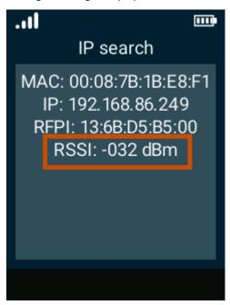
As you walk around with the wireless handset, the RSSI automatically updates onscreen with the signal strength for that area.
